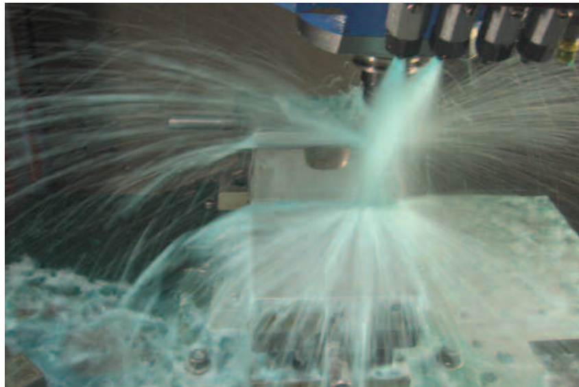
Ti-5553 Machinability Testing; Determining Range of Operating Parameters
