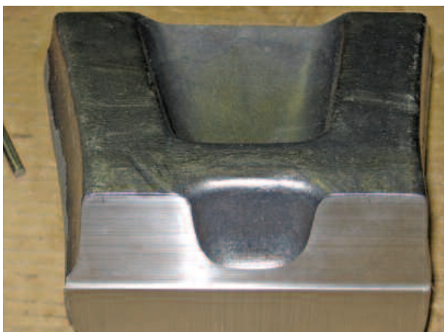
Ti-5553 Forging Sample; showing "skin" and as fixtured in Mazak milling machine for machinability testing
