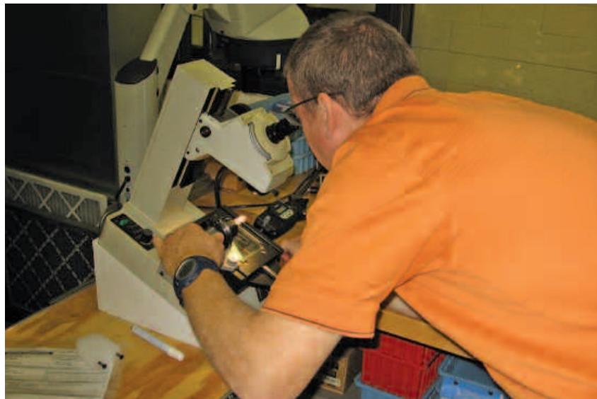
Yair Bruhis Monitoring Tool Wear During Machining Tests
