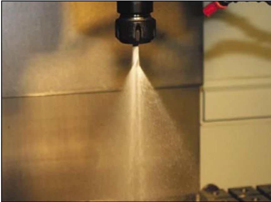
Use ER Coolant Rings without "o" ring for coolant surround tool application.
