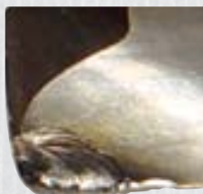
ER chuck wear detail
