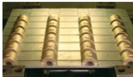
Laser-etching marks master collet pads in the B-pad cell at Hardinge.
