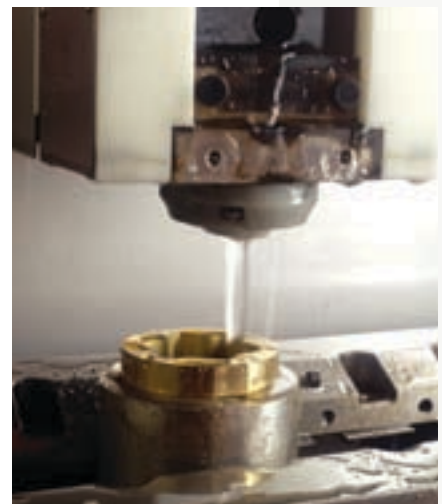
Special-shaped through-hole is being cut using a wire EDM (electrical discharge machine).
