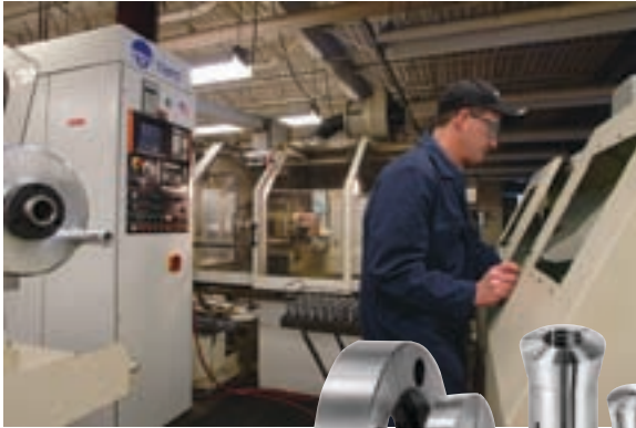
Precision grinding of the order hole takes place on a Tripet grinding machine in the 5C cell. Collets are then laser etched in the same work cell.
