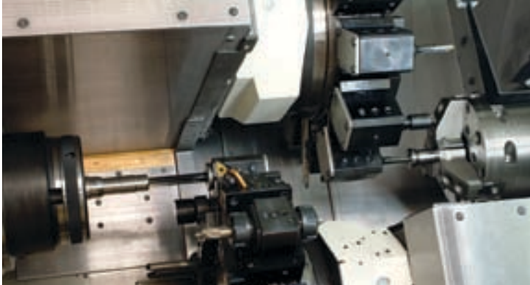
TSG-20R guide bushings are turned, threaded and bored on a Hardinge QUEST® TwinTurn® 65 twin-spindle, twin-turret CNC lathe with bar feed. Simultaneous machining is one of the many methods Hardinge uses to increase productivity.
