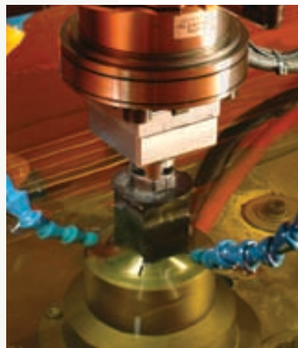
Submerged ram EDM (electrical discharge machining) removes material via an electrode – ideal for stepped-hole collets.
