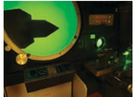
Hardinge checks the accuracy of the nose angle of a headstock center using an optical comparator measuring device.
